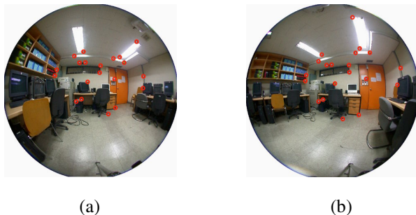
Fig. 1. Input images were taken by Nikon FC-E8 fisheye converter mounted on Nikon Coolpix995 with 1530 \times 1530 pixels and 20 correspondences marked by red circles. (a) omnidirectional image captured at the reference position, (b) at relatively rotated and translated position (rotation \mathbf{R} : -30^\circ around y-axis, unit translation vector \mathbf{T} : (t_x, t_y, t_z) = (0.9701, 0, 0.2425) ).
